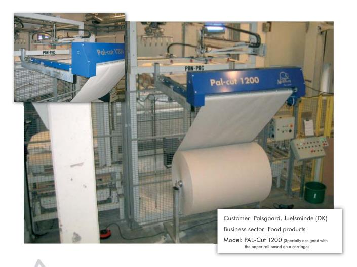
The customer had problems with the robot taking several sheets at a time as well as loss of sheets.
